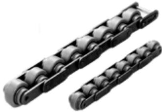
The chain speed is about 1/2.6 of the pallet carrying speed owing to special mechanism of the chain roller. Therefore, silent and smooth transportation is ensured. Accumulation of carrying materials can be performed smoothly since the main roller is set to free flow state. As the mechanism of the roller link constructs a basic bush press-in structure, the chain elongate-less and high-speed running can be performed.
