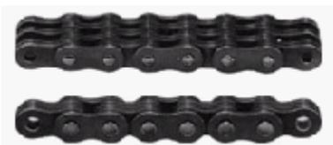
Interfaced plates held together by riveted pins. Use in applications requiring flexible linkage for reciprocating motion or lift. well suited for lift truck and counter weights.
