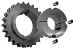
Off-the-shelf service complete with bushing for the desired shaft size can be provided with large range of Taper-Lock Sprockets. They are easily installed, removed and grip firmly, even on worn or under-size shafts
